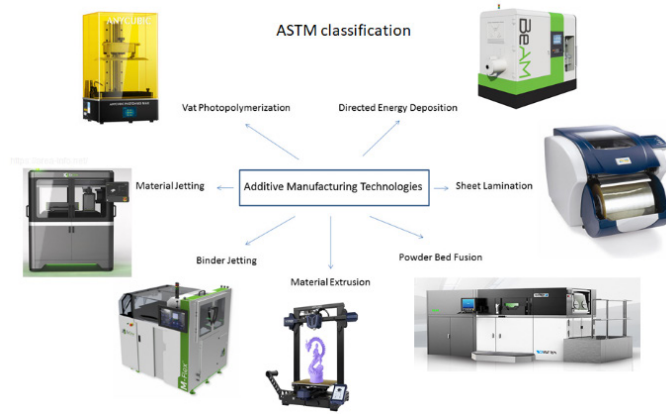
Figure 1. The seven categories of additive manufacturing given by ASTM F42.
