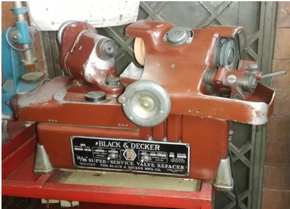
Figura 6. B&D 11/16" Valve Refacer.
